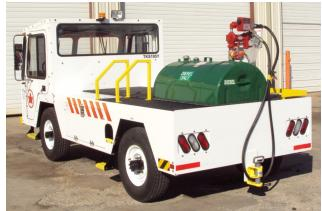
The GS500 is a high speed tow vehicle designed to meet a variety of needs in airline GSE applications.
